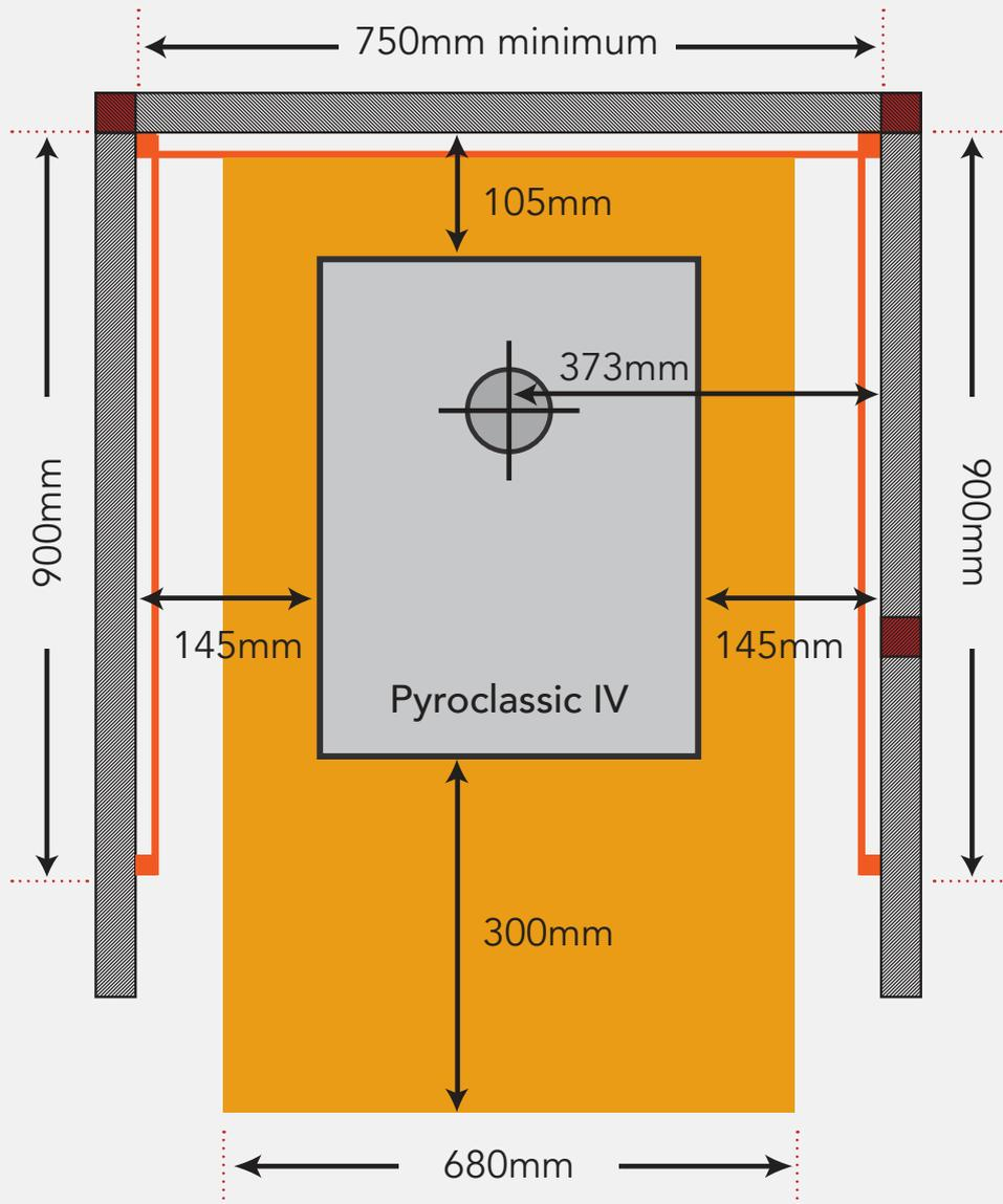
Side screens will only need to protect the combustible lengths of the built wall up to 900mm. If wall is shorter, the screen will be shorter.
